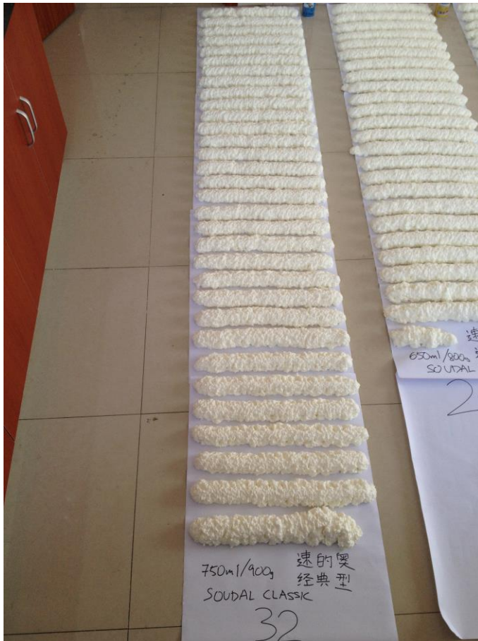
32 beads of foam from a single can of Soudafoam Gun, in their final, fully expanded state.
